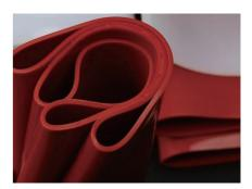
Silicone Rubber Silicone rubber itself has natural flame retardant properties, but its tearing performance is very poor. Micronized aluminum hydroxide can improve the tracking and erosion resistance of silicone rubber.
